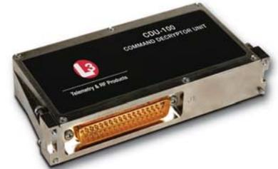
The Command Decryption Unit (CDU-100) is an integrated decryptor unit providing security capabilities for satellite communications links. The CDU-100 secures uplink data and provides command authentication in a small lightweight housing. The CDU-100 has 64 bits of telemetry data that reports health and status and is designed for missions up to 15 years. It supports data rates of up to 1Mbps utilizing 16 selectable keys.
